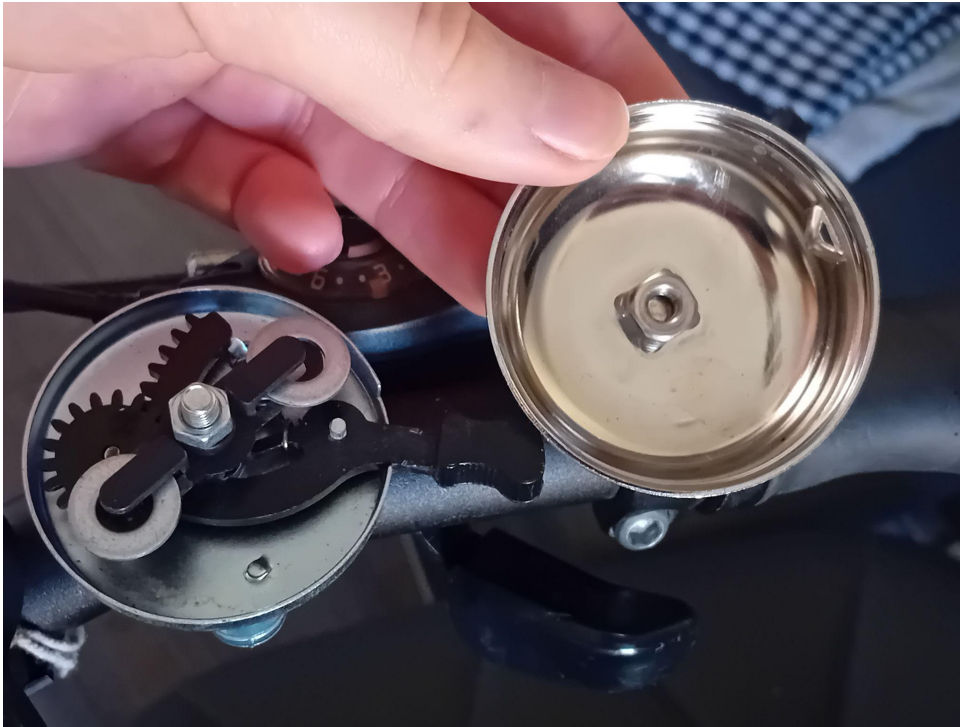
Figure 6.1.2. The internal mechanism of the multi-impulse bell. Also visible is the “bump” on the inside of the body of the bell.
