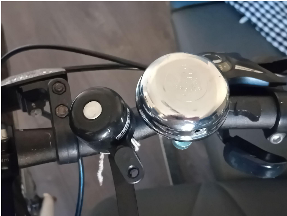
Figure 6.1.1. The two bells recorded for the study, mounted side by side on the handlebar of a bike. On the left is the single-impulse, and on the right is the multi-impulse.
